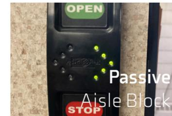
Requires the user to return to the open aisle keypad before opening a new aisle, ensuring the safety of other users.
