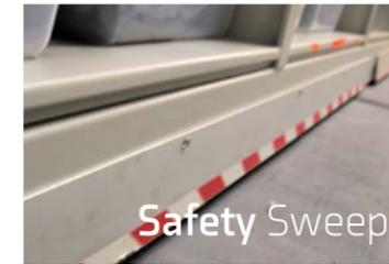
Designed to detect and clear obstructions from the path, our safety sweep ensures safe and reliable operation.
